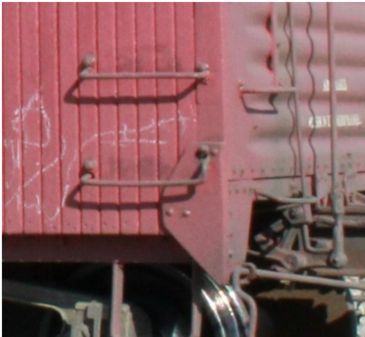
3. The lower door tracks for the Superior panel door are separate parts and fit on the cast on posts on the car side. The section of lower door track underneath the door is cast into the side and the separate track extends to the left of the door.
