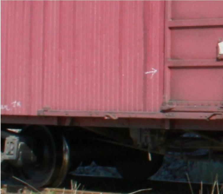
4. The opening and door latch lever must be added to the right side of the door.
