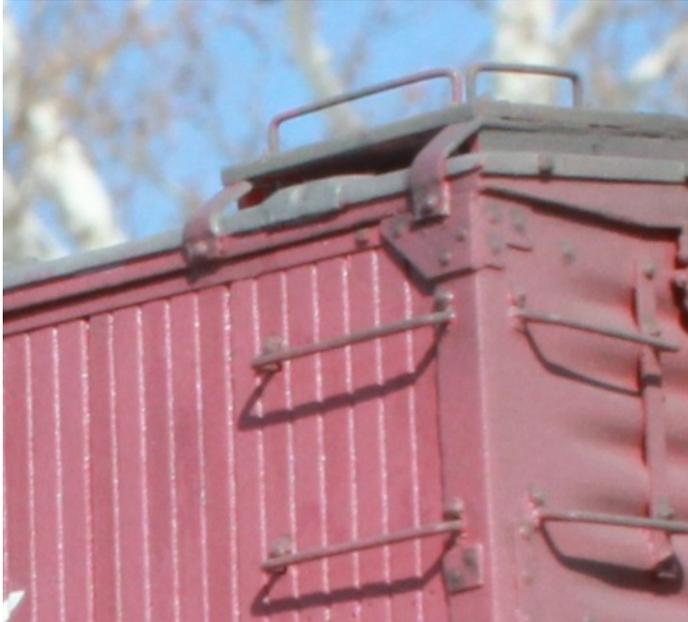
2. There are four larger gussets on the lower corners of the sides with the gussets on the right lower corner of the sides having a cast in grab iron end for the lowest grab iron on the side
